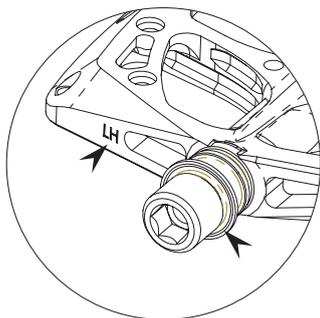
Identify right hand and left hand pedals by looking for the groove on the LH pedal spindle shoulder or the LH mark on the pedal body.
